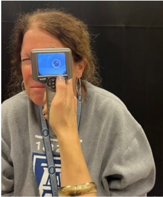
Figure 1. Procedure for measuring the pupillary light reflex variables.
