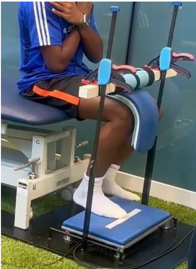
Figure 1. The test setting: force plate, adjustable bar, and appropriate padding.
