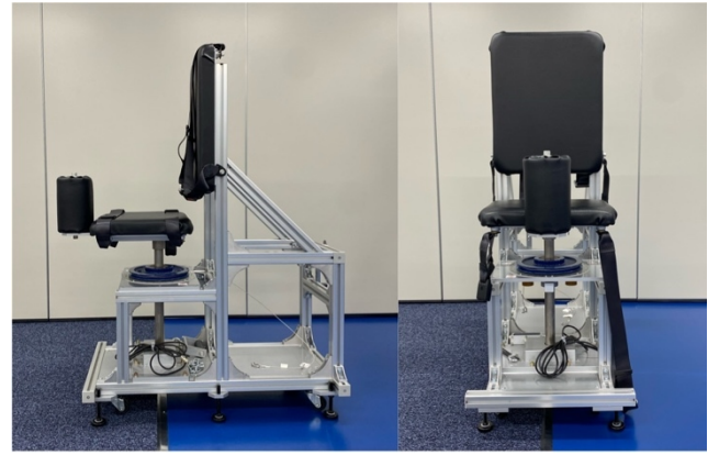
Figure 1. Lateral and frontal views of the trunk rotation dynamometer
