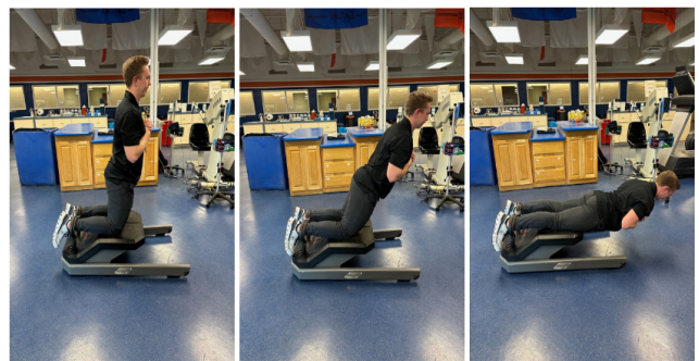
Figure 4. The eccentric hamstring curl test on the VALD NordBord device. The figure depicts the starting position (left image), the eccentric descent (middle image), and the completion of the test (right image)
