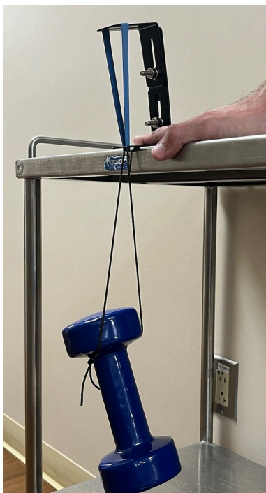
Figure 4. Measurement of the force required to stretch the 2 rubber bands by 5 inches.
