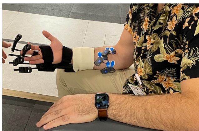
Figure 2. Finger flexor dynamometer in position for testing the middle finger in the long position.
