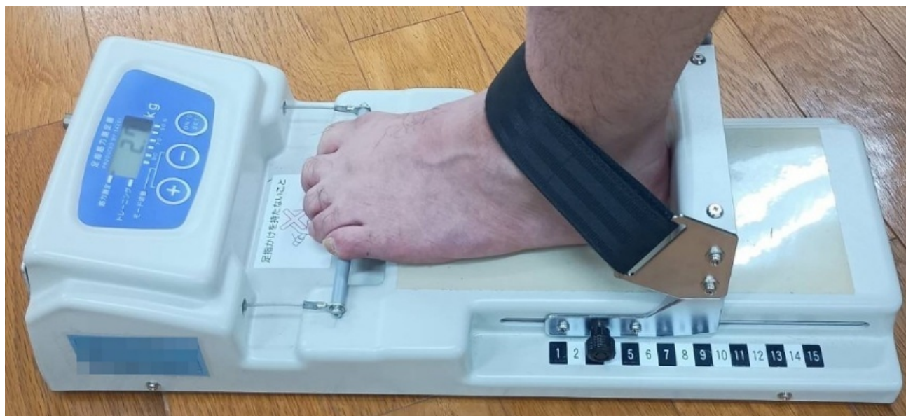
Figure 2. Toe-grip dynamometer used for measuring toe grip strength.
