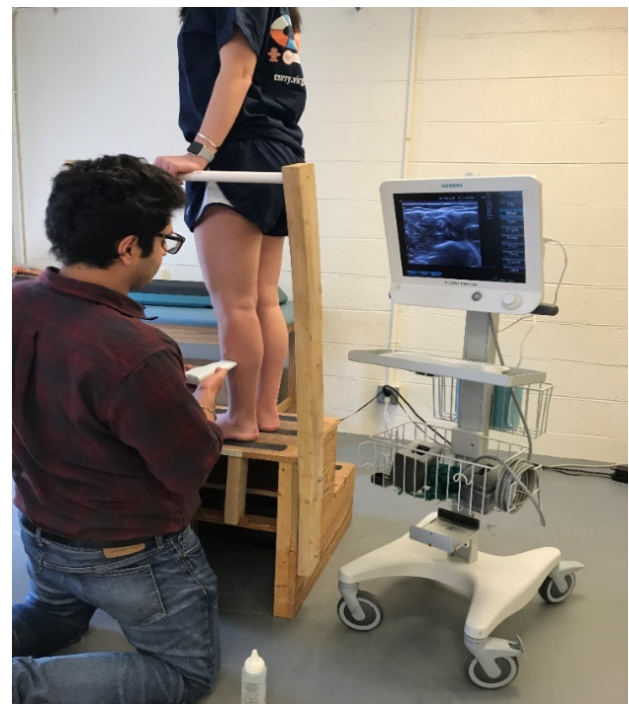
Figure 2. Customized step apparatus used for bipedal stance ultrasound imaging, with real-time image displayed on the ultrasound monitor.
