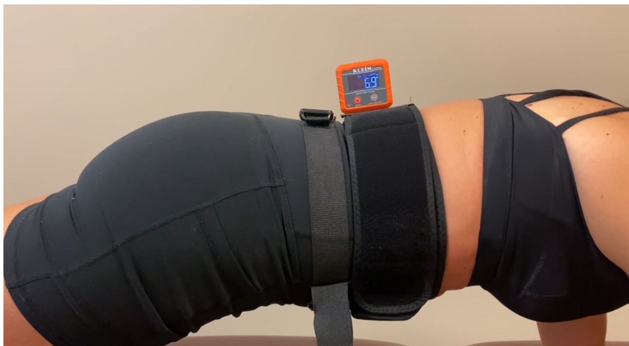
Figure 1. Experimental setup showing the digital inclinometer secured to the participant's trunk with a Velcro harness at approximately L4-L5.
